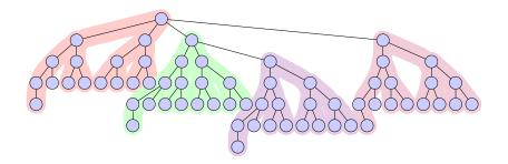
To map the hardware network hierarchy, two levels of trees are joined: In the example, *representative* processes of nodes (node0, node1, node2, node3) are interconnected following a *binary* tree, and processes belonging to the same node (16 process / node in this case) are also connected following independent *binary* trees.
